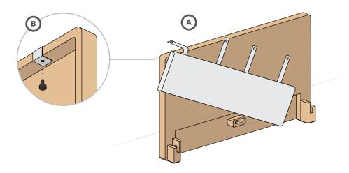
While holding the headboard slightly tilted inward, insert the long rail with "U" joint facing down and screws side facing inward.
