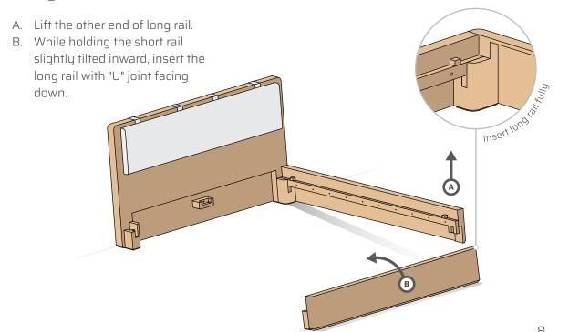
Place the remaining long rail into the headboard joinery and the short rail joinery, with "U" joints facing down. Press it down fully.
