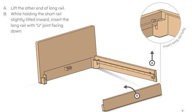
Place the remaining long rail into the headboard joinery and the short rail joinery, with "U" joints
