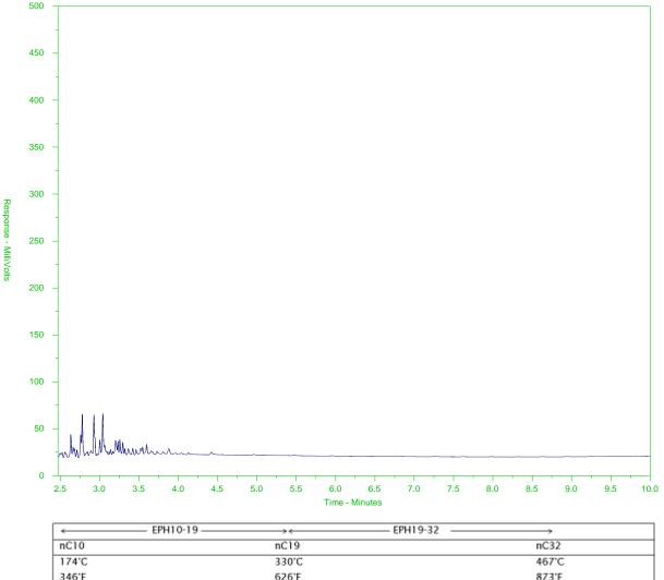
346'F 626'F 873'F ← Gasoline → Motor Oils/ Lube Oils/ Grease Diesel/ Jet Fuels
