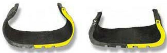
Normal Sidewall and Thick Run Flat Sidewall
