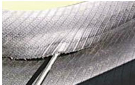
Bead Crack Inner (Bead Retak Bagian Dalam)
