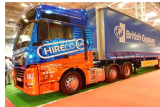
6 axle Artic 44 tonne GVW Curtainsider
