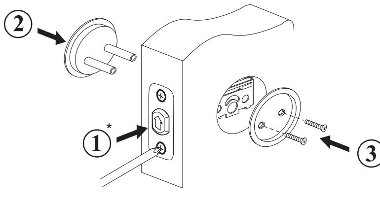
\*Proper installation allows the "thumb pull" to open from bottom, as shown.
