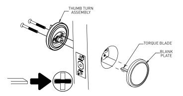
Insert torque blade horizontally into deadbolt latch. Crank until indicator assembly is flush with the door face. Mate the thumbturn assembly with the torque blade on the indicator assembly. Insert the screws through the holes of the thumbturn assembly and latch body. Tighten the screws to the threaded posts of the blank mounting plate. Tighten the assembly so the complete assembly is tight to the door.
