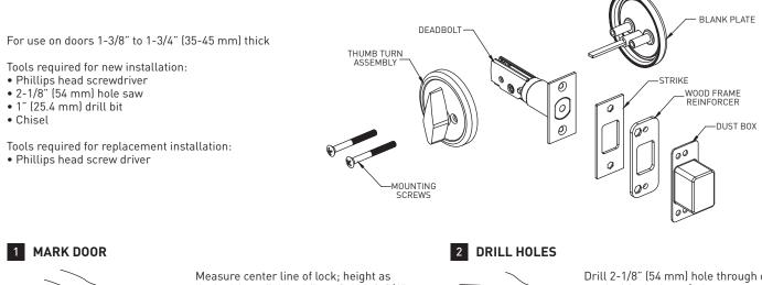
Measure center line of lock; height as desired from finished floor. Select 2-3/4" or optional 2-3/8" backset, fold and apply template to interior side of door and mark center of door as indicated on template. Mark center hole on door face through guide on template. Drill 2-1/8" (54 mm) hole through door face as marked for lockset. (It is recommended that holes be drilled from both sides on wood doors to prevent splitting.) Drill 1" (25.4 mm) hole in center of door edge for latch.
