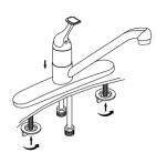
From under sink, thread mounting nuts (#15) onto bolts (#14) and tighten nuts.
