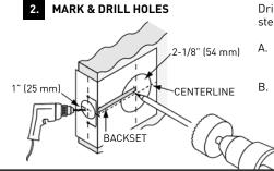
Drill 1/8" (3 mm) pilot holes as marked in previous step for both 1" (25 mm) and 2-1/8" (54 mm) holes.
