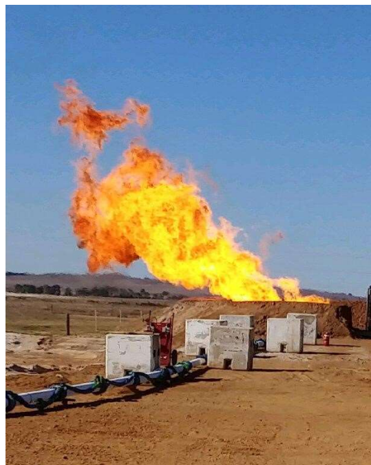
Figure 1 - flaring gas at surface on during D Sand testing
