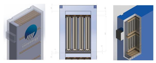
Figure 1 - Cross section of the ABS60 battery pack showing cell configuration
