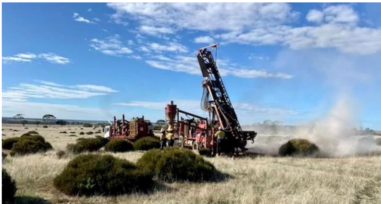
Figure 2: Drill rig currently drilling the first RC drill hole as part of the Phase III RC drill program at the Burracoppin Gold Project
