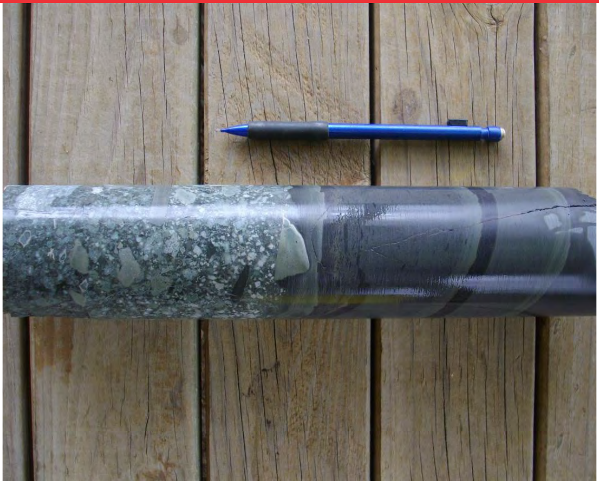
Figure 5.1_12 Drill Core – Diatreme Breccia intercepted in Hole RRD-01 (Source – Leached Cap, 2015)
