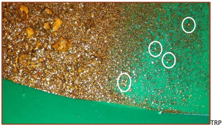
Figure 8. Crushed Iron pisolith sample containing gold grading up to 282 g/t in iron pisolites. (Source: TRP)
