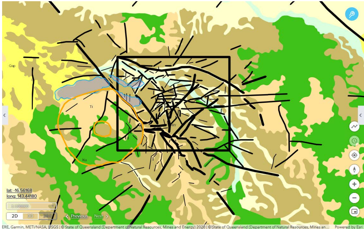
Figure 6. 1:100K GSQ Surface Geology. Overlain polygons (blue) represents mapped extents of outcropping felsic volcanic breccia and ignimbrite. Orange polylines represent sub-cropping (hypothesised) collapse cauldron with possible resurgent dome in centre. Black polylines are hypothesised sub-surface penetrative structures interpreted from combinations of remotely sensed data and field observations – particularly sub-surface influences on cover. The outcropping felsic volcanics may represent a partially exposed and structurally disrupted ring-dyke complex associated with collapse of the sub-circular feature. Landsat bands 7/6/2 and 5/6/2 highlight the outcrops and inferred sub-crops against the more extensive unconsolidated cover (Wyaaba beds and Bulimba formation) particularly well. (Source TRP).
