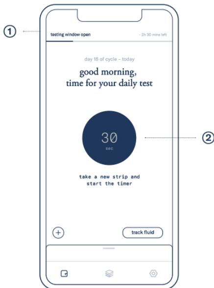
Once the testing window is open, it is displayed in a banner ① in the inne APP showing how much time is left to perform the test. The timer ② can be started from the 'lab' tab while the testing window is open.
