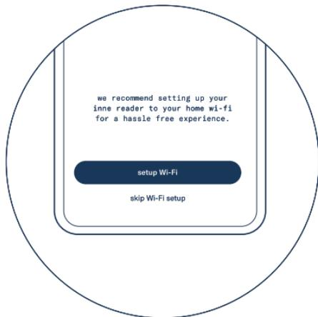
Setup a Wi-Fi connection for the inne READER after successfully pairing it with the inne account. Tap 'set up Wi-Fi' to start the process.
