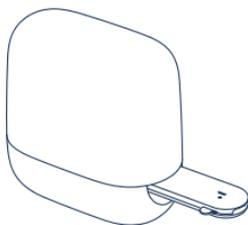
**CAUTION** The inne STRIP needs to be inserted into the inne READER right after it has been activated to ensure accurate results.
