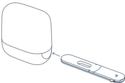
**TIP** Make sure to insert the window side of the inne STRIP first as shown and check that nothing is covering the strip window.
