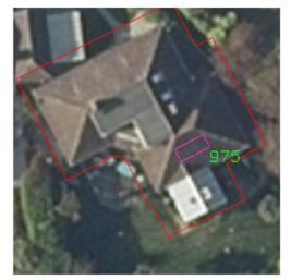
Small available roof area, only able to install <5 modules (<1.5 kW)
