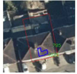
Radiation on east / west roof is insufficient, but high on the south-facing part
