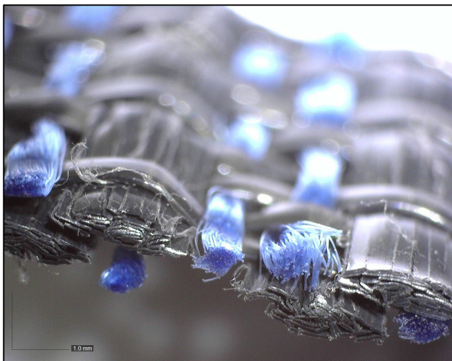
Figure 1. Close-up of H 2 Ri (Black polypropylene yarn for reinforcement and stabilization and blue textured yarn for moisture management) (source: Solmax).
