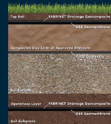
Municipal Waste Landfill with Geosynthetics
