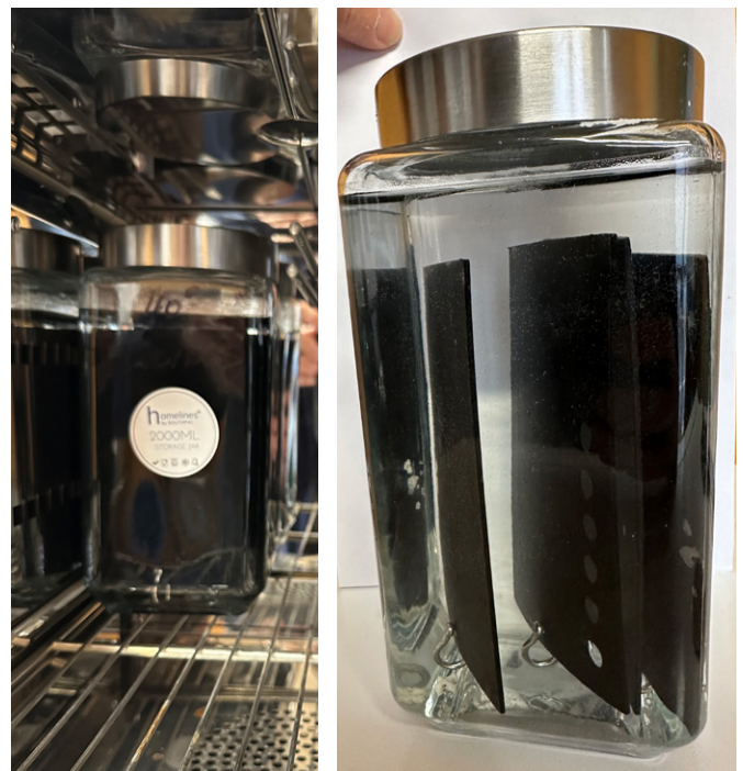
Figure 1: The immersion apparatus: GSE HX samples immersed in 40 C brine solution
