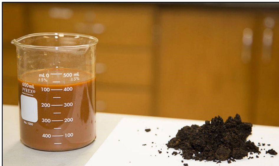
Figure 6 AMD clarifier slurry @ 2% solids versus 65% dry solids from inside geotextile tube
