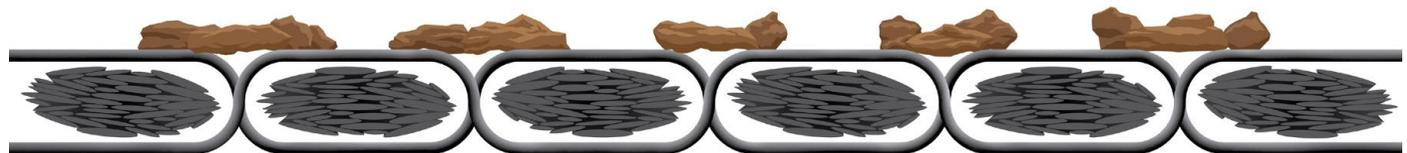
**A standard single layer geotextile has a smoother surface, providing less opportunity for soil interaction**
