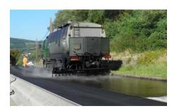
Spraying of tack coat should always be undertaken using a truck-mounted calibrated spraying-bar to ensure the correct quantity is applied. The tack coat should be sprayed 15 cm wider than the width of the **MIRAGRID** PGL.
