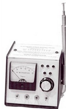
Figure 5. Illustration of the Yeaple Probe.
