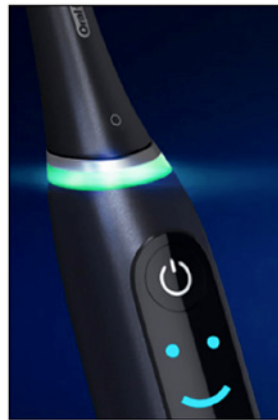
Figure 7b. Pressure sensor light illumination – correct pressure.
