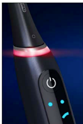
Figure 7a. Pressure sensor light illumination – too much pressure.
