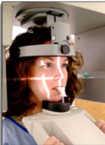
Figure 18. Panoramic unit (OP100, Instrumentarium Imaging) with light beam reference guides projected onto the patient's face to help the clinician align the head.
