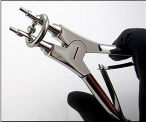
Figure 27. Ring expanding pliers being used to expand ring.
