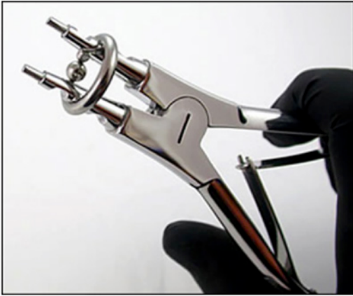
Figure 28. Ring expanding pliers being used to expand ring.
