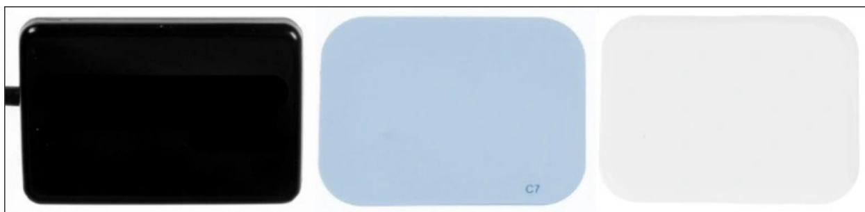
Figure 1: Rigid CCD Digital Sensor
