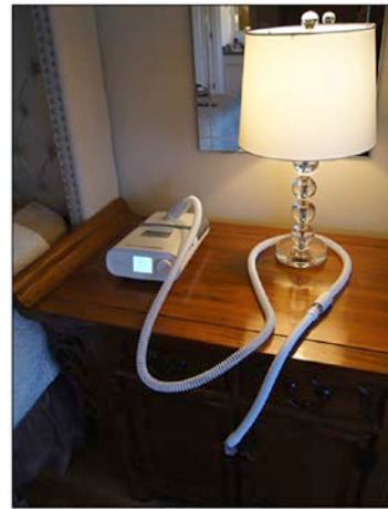
Figure 5. A typical set up of a bedside, home-use positive airway pressure (PAP) unit. The proximal tubing connects to the device, in this case it is attached to the humidifier portion of the PAP. The distal end will be fitted to the patient's mask.
