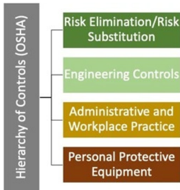
Figure 2. OSHA's Hierarchy of Infection Controls in Healthcare Environments
