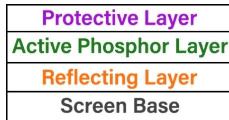
Figure 8. Intensifying Screen. Diagrammatic cross-section of screen
