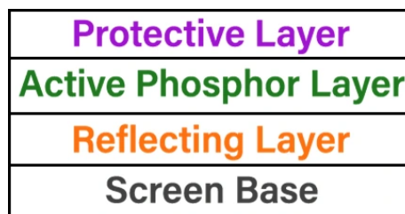
Figure 8. Intensifying Screen. Diagrammatic cross-section of screen
