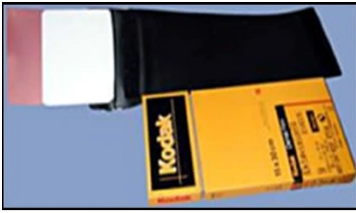
Figure 10. Flexible Cassette with Panoramic Film. Partially open flexible cassette showing screen (white) and film (purple) surfaces.
