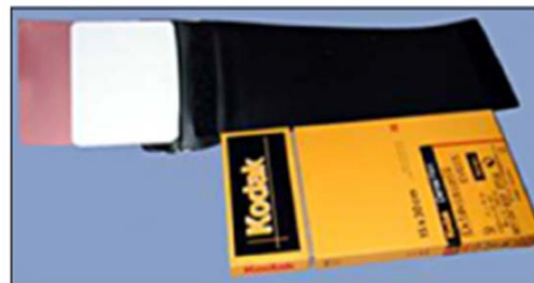
Figure 10. Flexible Cassette with Panoramic Film. Partially open flexible cassette showing screen (white) and film (purple) surfaces.
