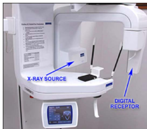
Figure 2. Digital Panoramic X-ray Unit. Source: 2009 Proline Panoramic XC, Planmeca
