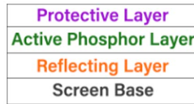
Figure 8. Intensifying Screen. Diagrammatic cross-section of screen
