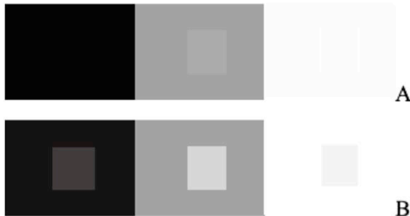
Figure 6. Comparison of 2 systems. In each rectangle, there is a square that has a grey value close to the grey value of the rectangle. A has a low contrast resolution. B has a high contrast resolution.
