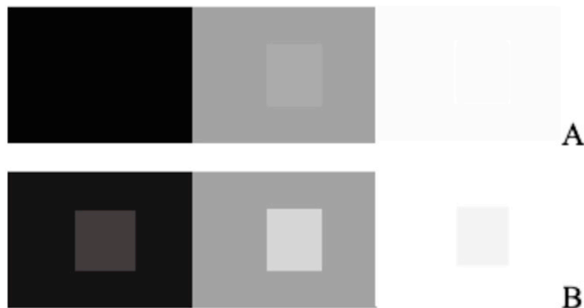
Figure 6. Comparison of 2 systems. In each rectangle, there is a square with a grey value close to the grey value of the rectangle. A has a low contrast resolution. B has a high contrast resolution.
