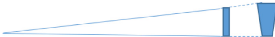
Figure 10. Distortion of the shape of the rectangle due to a change in the angle of incidence of an x-ray beam.
