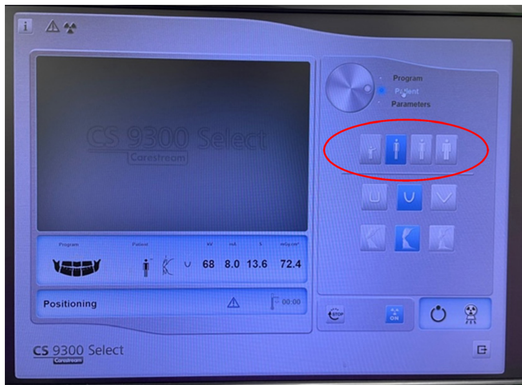
Figure 4. Sample screen for selecting exposure settings for a child, slender adult, average adult, and large adult (circled in red). It is currently set for a slender adult with a curved arch.
