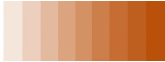
Fig. 6b - Chroma increases from left to right, while value decreases in the same direction.
