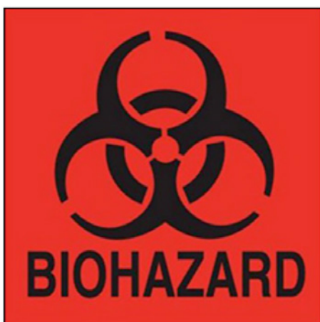
Figure 7. The universal biohazard label must be fluorescent orange or orange-red, with lettering and symbol in a contrasting color.
