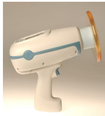
Figure 6. Handheld Intraoral X-ray Device
