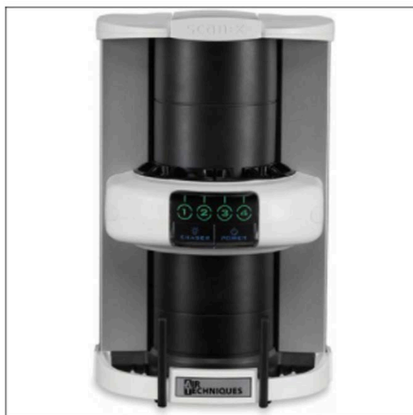
Figure 8. Indirect Photo-stimulable Phosphor Imaging System.
