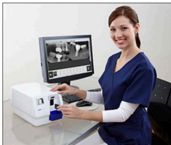
Figure 9. Indirect Photo-stimulable Phosphor Imaging System.
