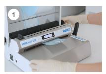
Cut three 10 cm test strips from the smallest packaging format used in the practice.
