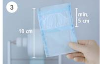
All test strips must have two seal seams separated by a gap of at least 5 cm.
