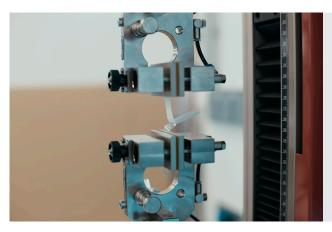
The seal seam stability test is a standardized test procedure and represents a part of EN ISO 11607-2 for the validation of packaging processes. The annual routine check of the sealing seam stability serves the performance qualification (PQ) of MELAG sealing devices and is carried out according to EN 868-5.
