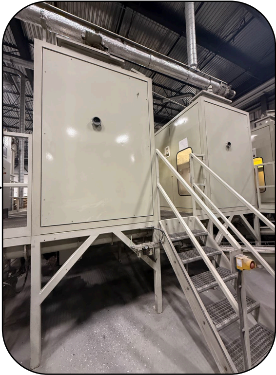
Electrostatic Separator ABS from HIPS
