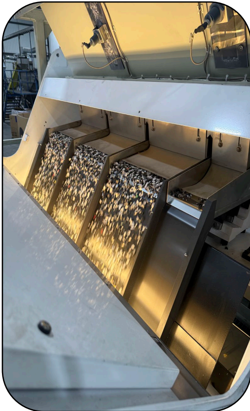
Rubber Sorter Removes rubber, wood, foam
