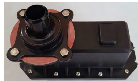
Install Meter-Funnel and Gasket
