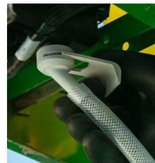
Install Quick-Attach Latch
