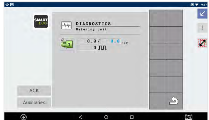
Diagnostics Screen - Metering Unit
