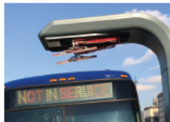
Figure 1. J-3105-1: Infrastructure-Mounted Cross Rail Connection
