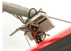
Figure 2. J-3105-2: Vehicle-Mounted Pantograph (Bus-up) Connection
