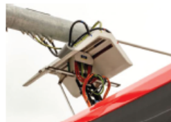
Figure 2. J-3105-2: Vehicle-Mounted Pantograph (Bus-up) Connection
