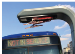
Figure 1. J-3105-1: Infrastructure-Mounted Cross Rail Connection
