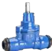
Series 03/30 Service connection valve with tensile socket ends for PE pipes DN20-50 PN16 Ductile iron
