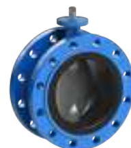
Series 75 Butterfly valve Centric with fixed liner Double flanged short DN50-2000 PN10/16 Ductile iron
