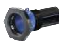
Series 635/00 Supa Maxi™ universal tensile transition coupling with factory mounted PE pipe DN50-300 PN10 or 16 Ductile iron
