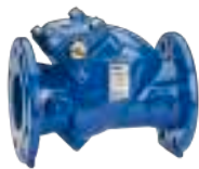
Series 41/60 Swing check valve Free shaft Resilient seated DN50-300 PN10/16 Ductile iron Options: • lever and weight • lever and spring • prepared for limit switch
