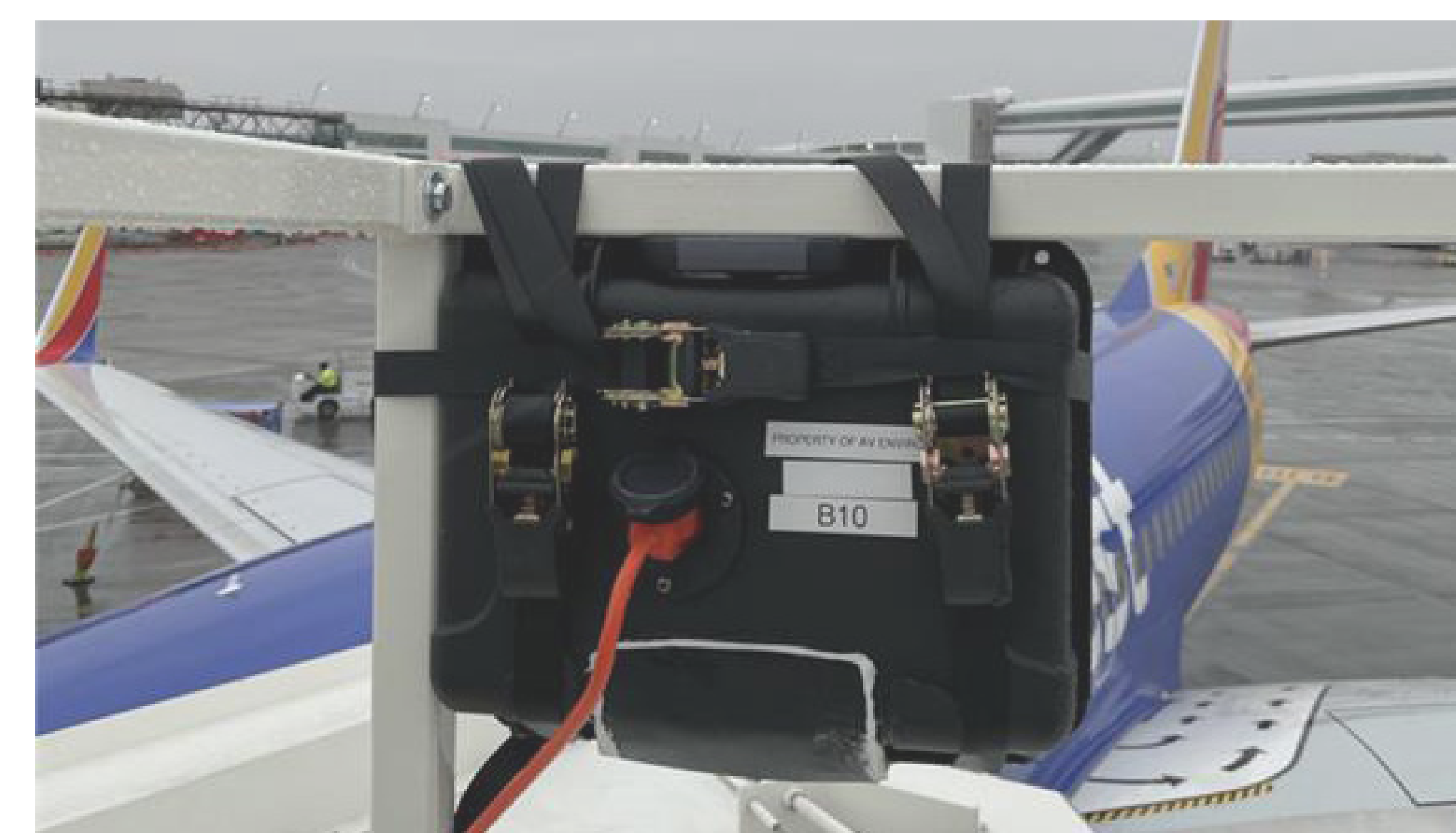
APU detection device installed at gate B10. All data is fed through our backend and displayed on our dashboard in real time
